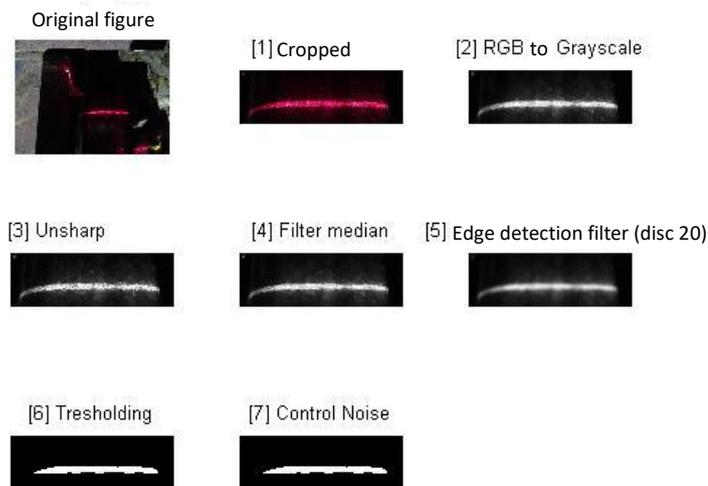
Figure 5. Result of each image processing from the original figure to control noise
