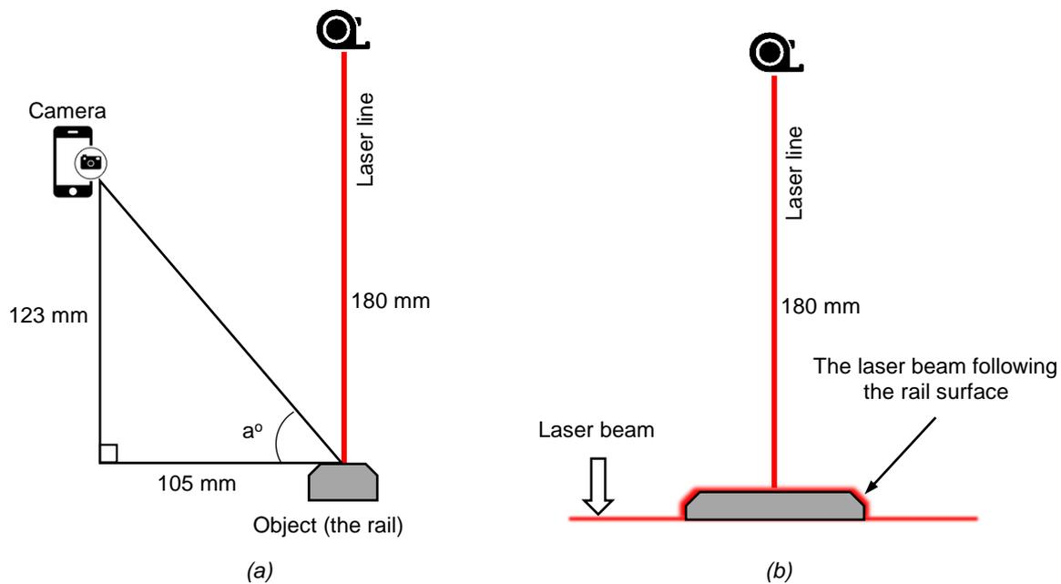
Figure 1. Camera and laser position toward the rail. (a) Side view. (b) Front view of rel
