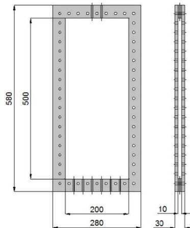
Figure 1. Dimensions of Helle Shaw Cell
