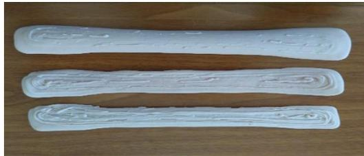
Figure 1. Specimen according to ASTM D638 Type 1.
