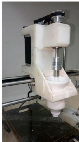
Figure 2. ASTM D638 Type 1 3D Printing Tool. Specimen Printing
