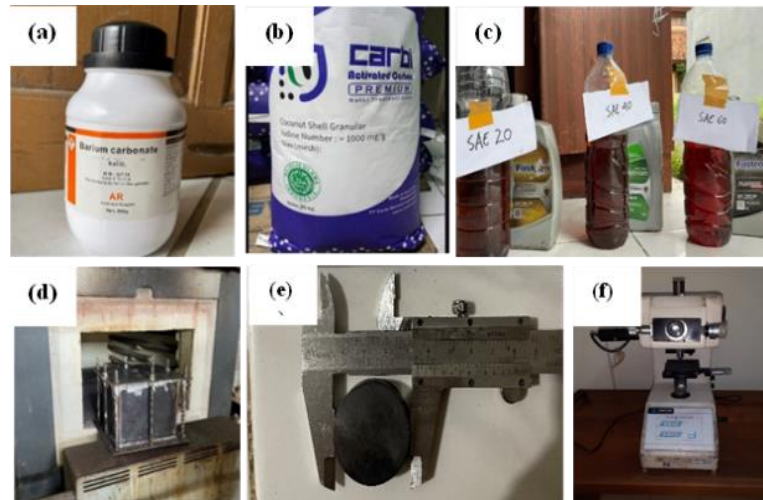
Figure 1. Tool of Carburizing Process: (a) Barium Carbonate ( BaCO_3 );(b) Coconut Shell Charcoal; (c)Cooling medium; (d) Pack carburizing; (e) Vernier Calliper;(f) Microvickers hardness tester
