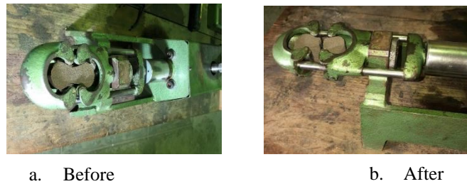
Figure 3. Tensile Test of Sand Specimens
