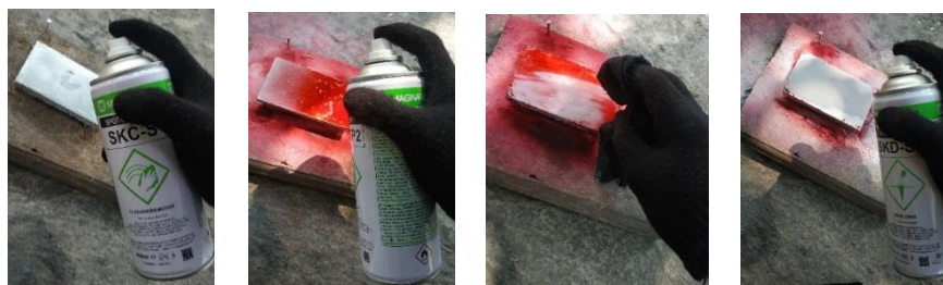
a. Cleaner spraying b. Red Penetrant spraying c. Red Penetrant wiping d. Developer spraying
