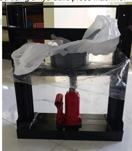
Figure 7. Composite pressing process with a hydraulic press machine
