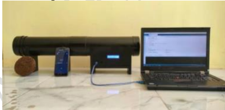
Figure 8. Test Equipment (Impedance Tube)
