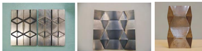
Figure 2. Construction of Origami Pattern Crash Box by stamping method [7]
