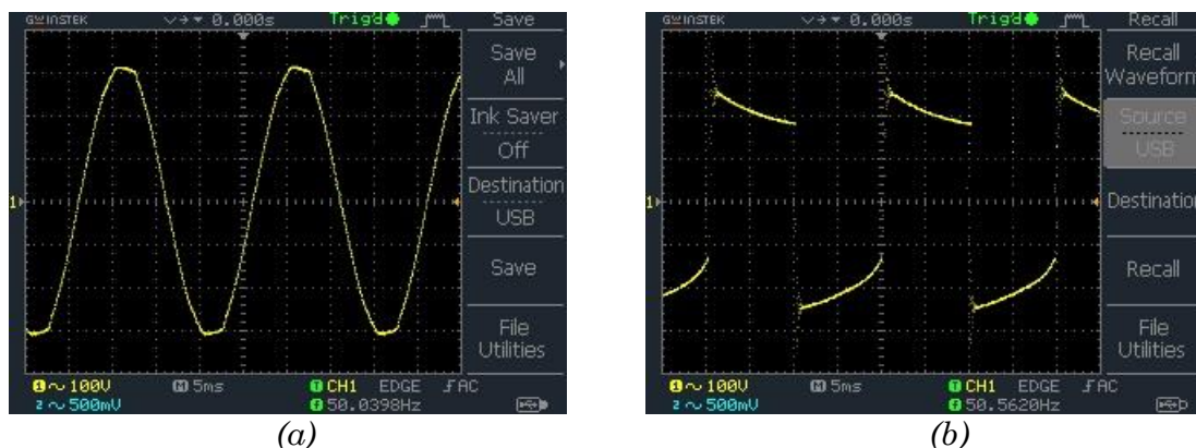
Fig. 10. The sinusoidal waveform of: (a) electricity grid, and (b) inverter output
