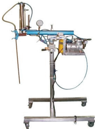
Figure 1. Fluidity test apparatus Vacuum Method
