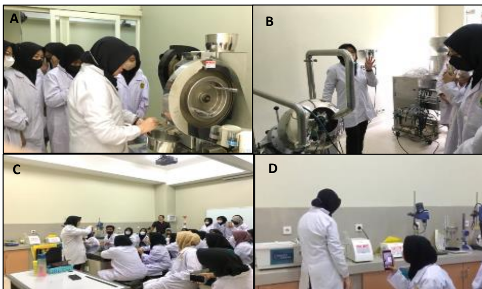
Figure 3. A and B. Practical simulation of tablet printing machines (Eccentric Desktop Type Press). C. Practical Simulation of the Disintegration Tester tool. D. Practical Simulation of Hardness Tester and Friability Tar (Tester) tools
