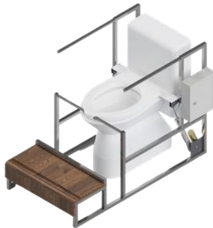
Figure 5. Finished design of elderly-friendly hydraulic toilets
