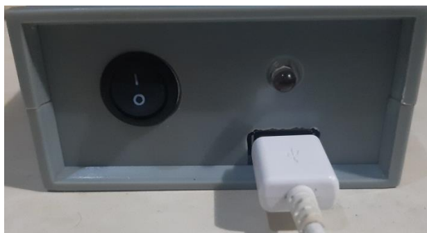
Gambar 8. Tombol Emergency, Lampu Indicator dan USB
