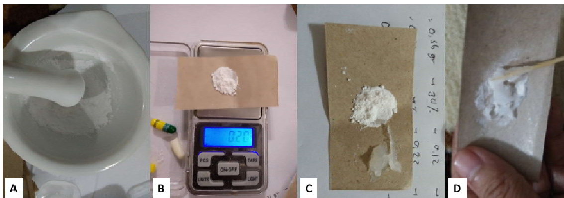
Figure 2. The tested drug formulation. The medicine to be tested is first mashed into homogeneous powder using a pestle and mortar (A) then all the medicinal powder preparations are weighed on a microgram (B) scale. About 30% of the powder was then taken and mixed with white paraffin using a toothpick (C and D).
