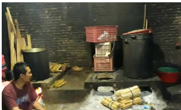
Figure 1. The use of a wood-fueled furnace in the steaming process
